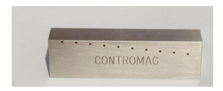
TEMOIN A is an excellent mean to check the polarity of the magnetizing coils as well the efficiency of the longitudinal magnetization.
